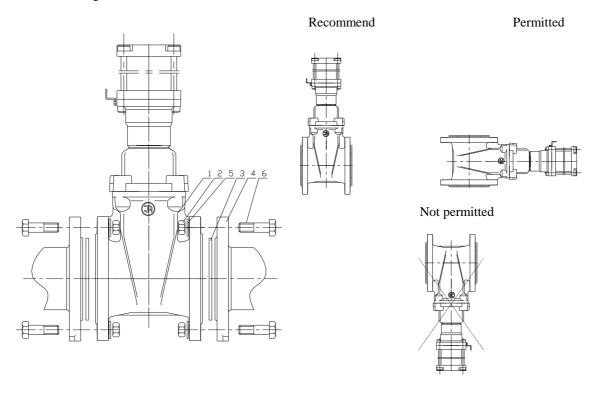
1. Valve; 2. Nut; 3. Gasket; 4. Pipeline flange; 5. Washer; 6. Fastening bolt
