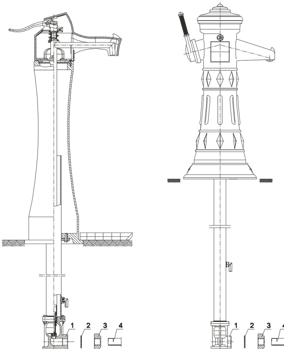
1. — hydrant, 2. — seal, 3. — pipeline connecting flange, 4. — pipeline
